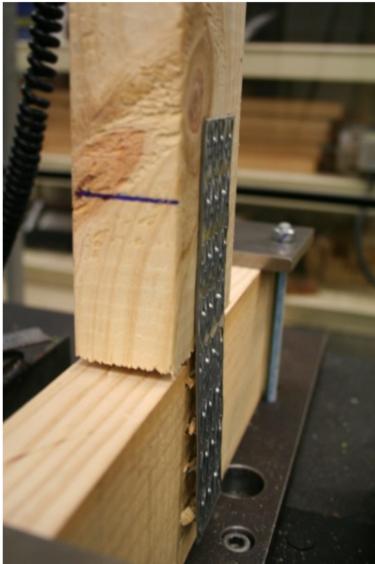
Figure A83 Typical mode of failure, pull-out of teeth from timber for perpendicular direction tests.
