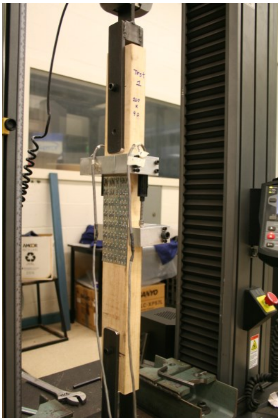
Figure A82 Typical test set-up for parallel type testing
