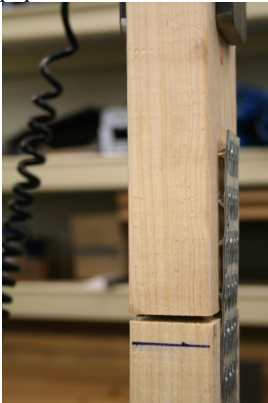
Figure A84 Typical mode of failure, pull-out of teeth from timber for parallel direction tests.
