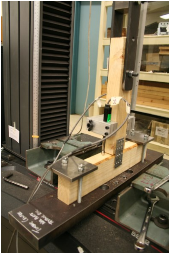
Figure A81 Typical test set-up for perpendicular type testing.
